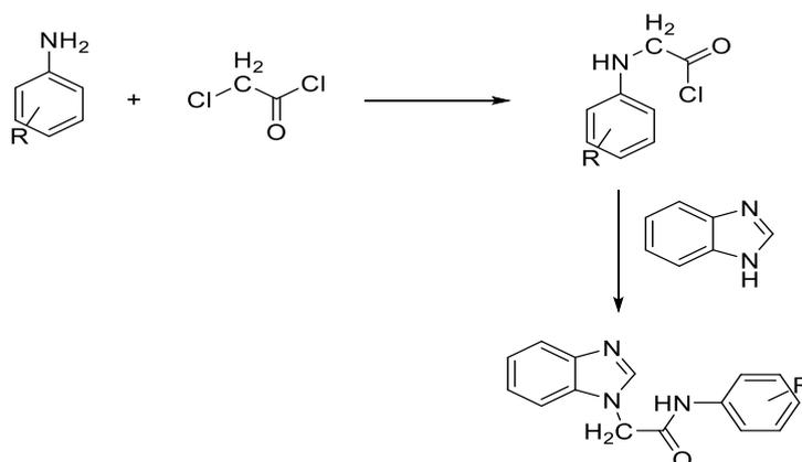
**Figure 6.** Synthesis of acetamide linked benzimidazole with a substituted phenyl ring
