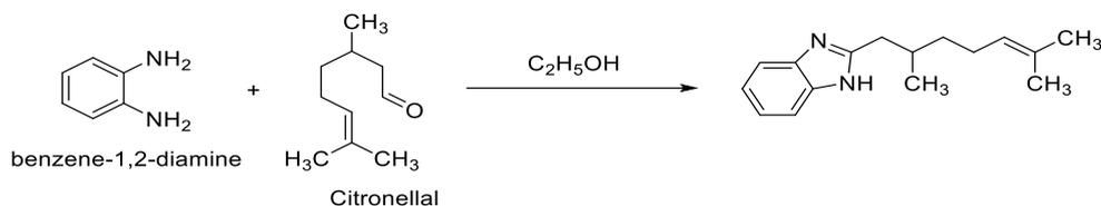
**Figure 5.** Synthesis of benzimidazole from Citronellal and *o*-phenylenediamine
