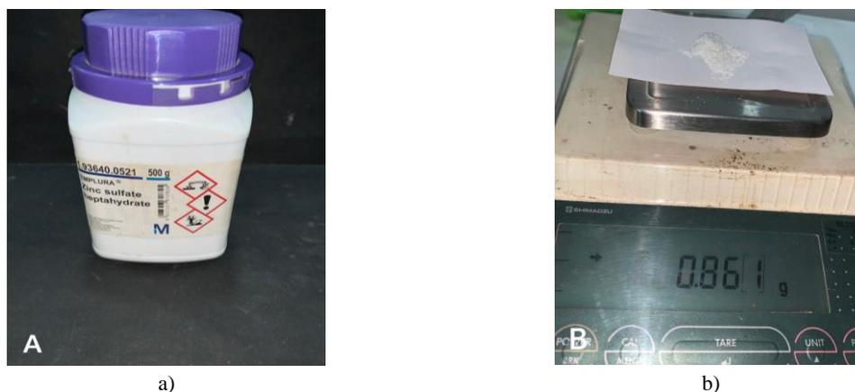
**Figure 3.** Image A depicts the zinc oxide powder. Image B depicts 0.861gms of zinc oxide that was measured to prepare the nanoparticle.
