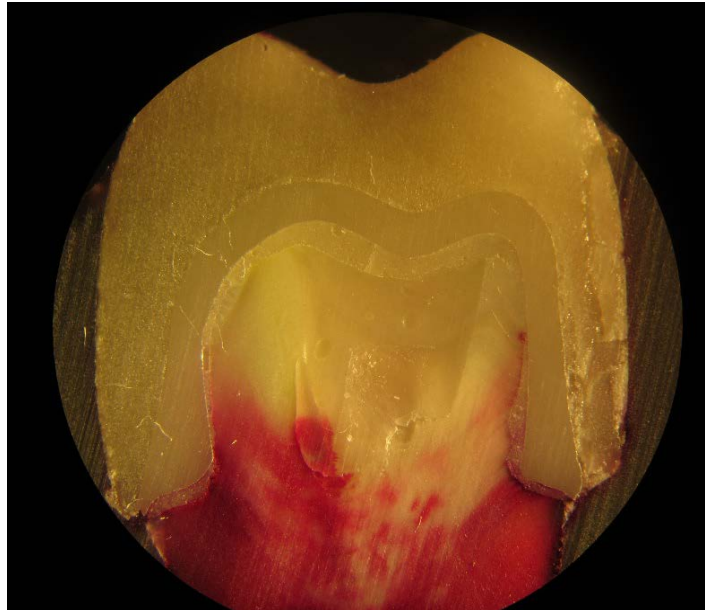
Figure 2. A sample with score 3 in dye penetration evaluation
