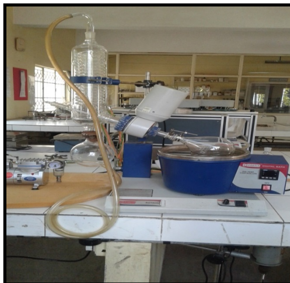
Figure 2: Rotary Evaporator Instrument used for Formulation and development of liposome
