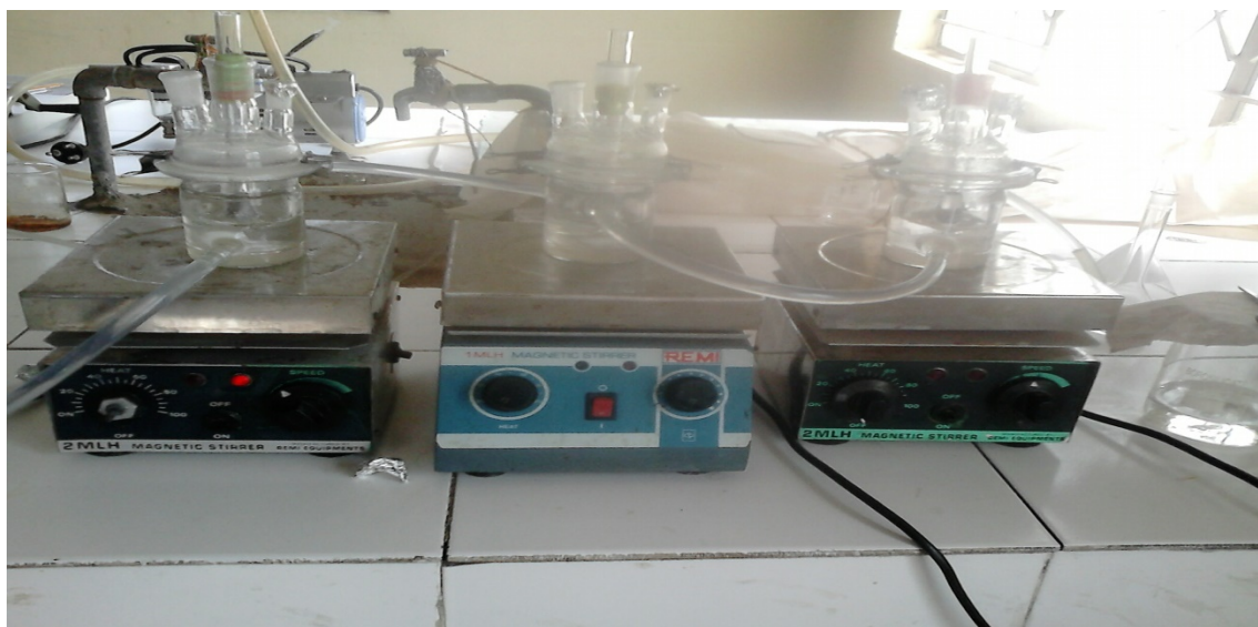
Figure 3 : Nasal diffusion cell assembly used in experimental work for drug release study
